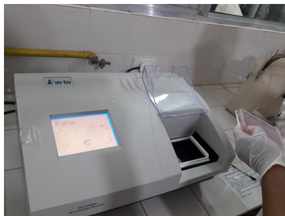
Figura Nro. 20: Lector de Elisa a 490 nm (Rayto RT-2100C Microplate Reader)
