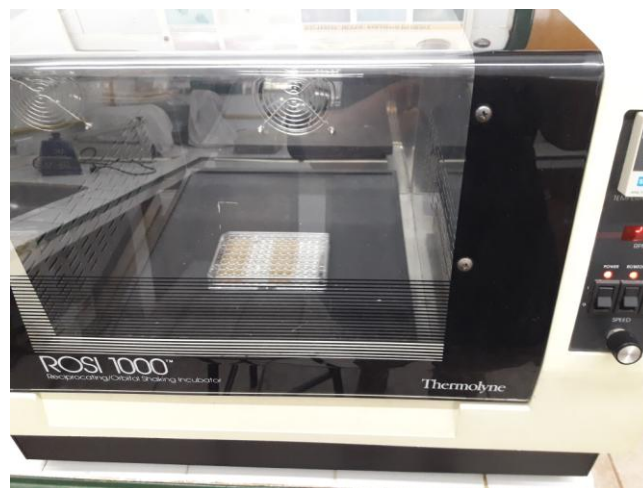
Figura Nro. 19: Incubadora con agitación orbital (Thermolyne ROSI 1000 Reciprocating Orbital Shaking Incubator)
