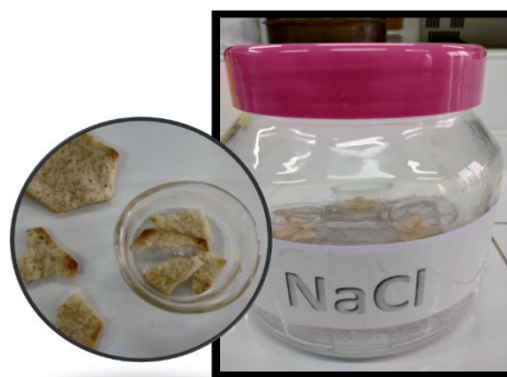
Figure 1: Methodology used for the determination of equilibrium moisture content.
