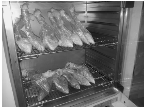
Figure 1. Small-scale plastic bag-based mass production of B. bassiana and M. anisopliae .
