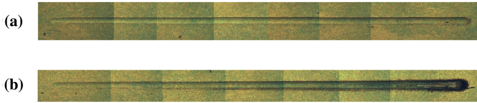
Fig. 2. Scratches produced on two coatings oxidized in 1 M solution of sulfuric acid at 40 V and 500°C: (a) without heat treatment, load of 2 N/mm, no failure; and (b) with heat treatment at 500°C, load of 4 N/mm, failure. Load increases from left to right.
