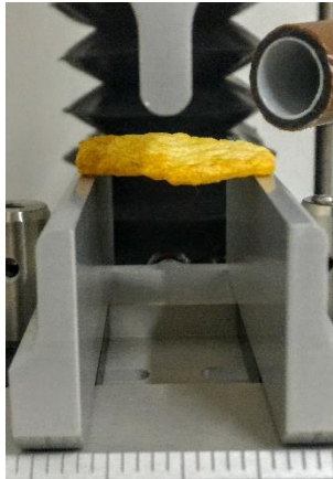
Figura 92 ensayo Three point bend (TPB)
