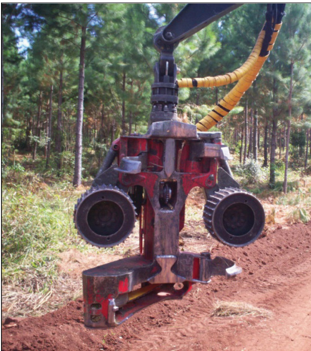
Figura 2. Cabezal procesador. Figure 2. Harvesting head.
